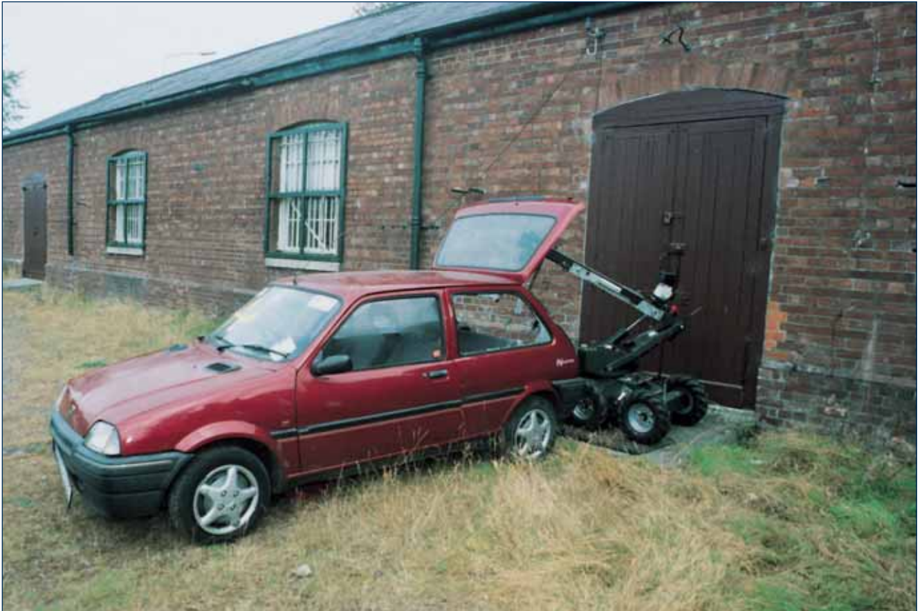
Scenario: suspect car with bomb reversed up to Dublin hotel. The HOBO robot is ideal for these situations.
